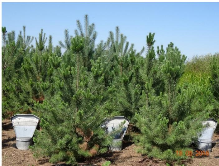
Fig. 1. Soil evaporimeters installed in compact enclave of Scots pine in field experiment
